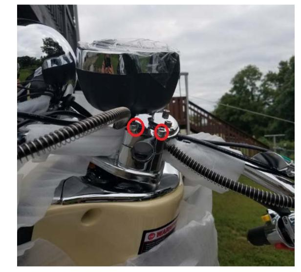
1, Remove these clamp bolts on the handle bar on both sides circled in red, should be 4 bolts (should be a 10mm socket size).
