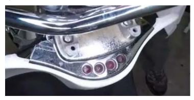
4, Put the top clamp block back on and screw the bolts in, but do not tighten down all the way, just tighten enough so that the handle bar will move a little so you can position it comfortably for you to ride.
