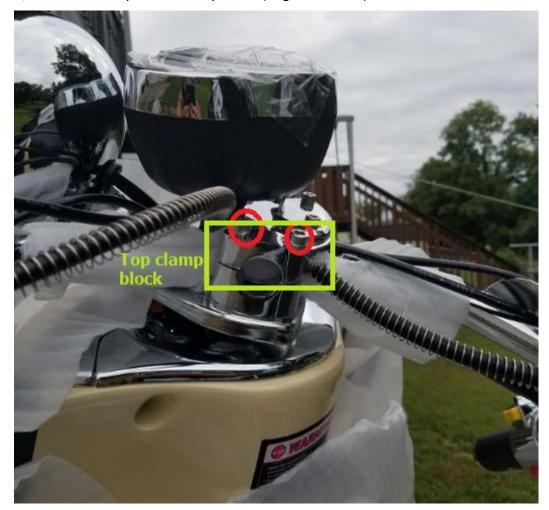
2, Remove the top to the clamp block (in green below)
