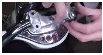
5, Put the handle bars in a position that is comfortable for you to reach and drive, tighten the bolts down tight enough so that your handle bar does not move. That's it!
